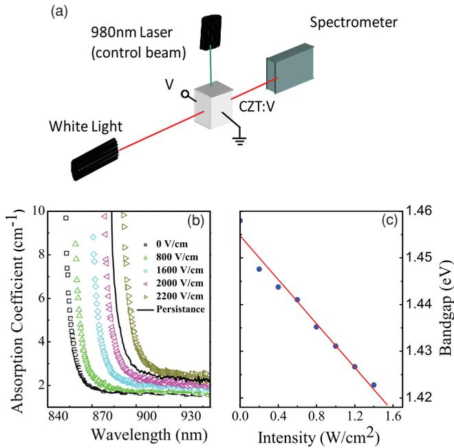
FIG. 1. (Color online) Experimental setup and experimental results demonstrating light-induced shift of the absorption edge of CZT:V crystals. (a) Setup. (b) Shift of the absorption spectrum as a function of applied field (at  $I_l = 1.3 \text{ W/cm}^2$ ). (c) Shift of the band-gap energy as a function of the control-beam intensity (at  $E = 1.8 \text{ kV/cm}$ ). Blue solid circles are the experimental data and the red solid line is the linear fit.
