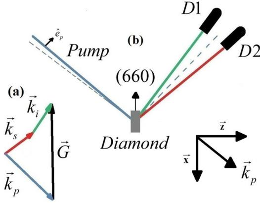
FIG. 1. (a) Phase-matching scheme. (b) Schematic of the experimental setup. The indices  $p, s$ , and  $i$  are for the pump, signal, and idler, respectively,  $\vec{G}$  represents the reciprocal lattice vector orthogonal to the (660) atomic planes, and  $\hat{e}$  is a polarization vector.  $D1$  and  $D2$  indicate the two detectors.
